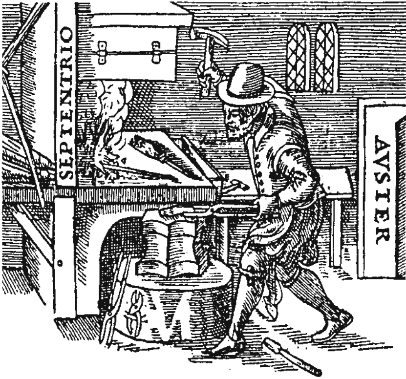
Fig. 1.1. Coldworking of a permanent magnet in the direction of the earth's magnetic field (septentrio=north, auster=south) taken from Gilbert [6]
